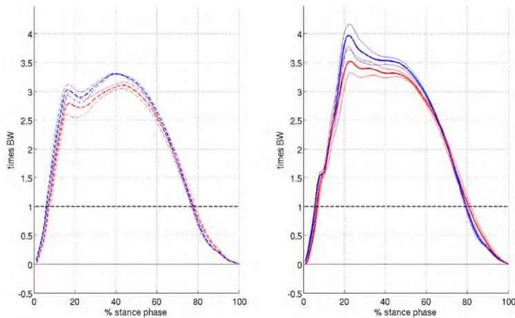
**Caption:** Mean vertical GRF (GRF<sub>z</sub>) in times BW plotted over % of stance phase, thick: mean, thin:  $\pm$  SD, left: 5.4m/s, right: 8m/s, blue: left foot, red: right foot
